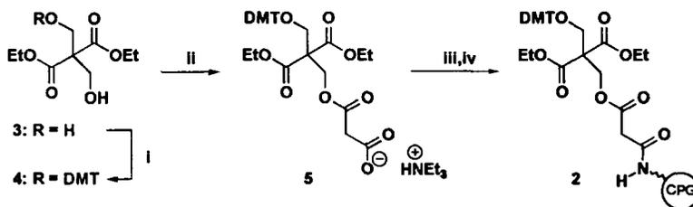
**Scheme 1** i: DMT-Cl/Py; ii: malonic acid/DCC/Py; iii: H<sub>2</sub>N-CPG/DIC/Py; iv: Ac<sub>2</sub>O/*N*-methylimidazole/Py/THF.
